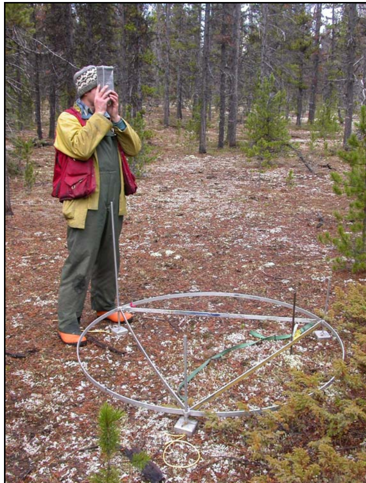
Figure 4. Moosehorn measurement of canopy cover over the plot.
