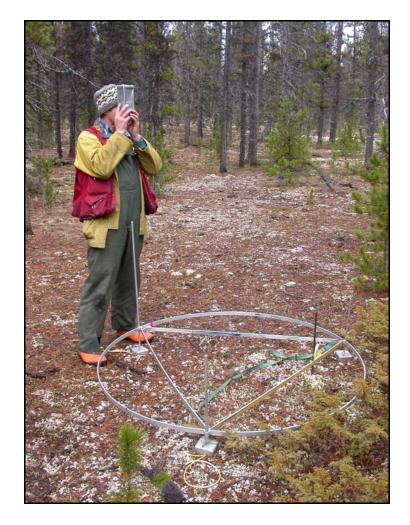
Figure 5. Moosehorn measurement of canopy cover over the plot.
