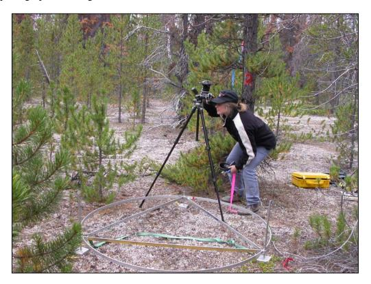
Figure 8. Taking canopy photos with a fisheye lens.
